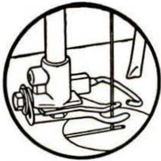
Blade guide aids close following of a line or pattern.
